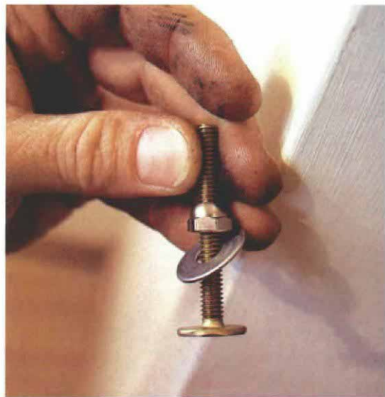
5. Closet bolts are made of brass and have machine threads and a T-shaped head. The head fits into the slot in the flange ring, and the bolt slides into position. Then, the head is turned 90°, and the bolt is tightened in place.
