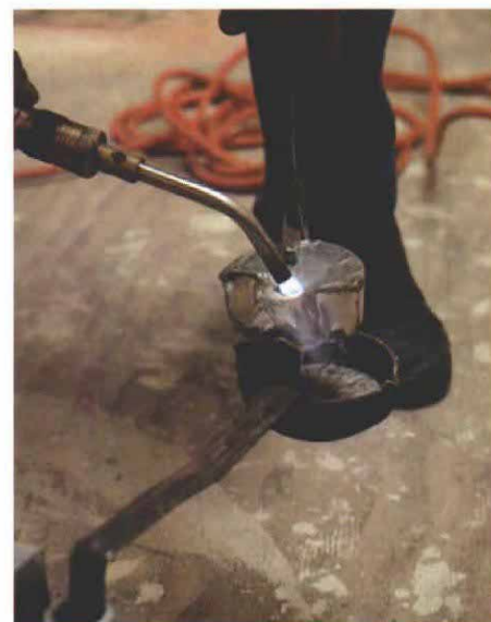
7. A bent-handled ladle, anchored by a box full of pipe nipples, makes a handy basin in which to catch molten lead.
